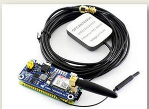
Figure 4. GSM Module
